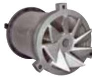
Cenpeller™ technology improves circular flow—forcing the debris to lay up against the surface of the strainer element in a way that makes backwashing easier and more efficient.
