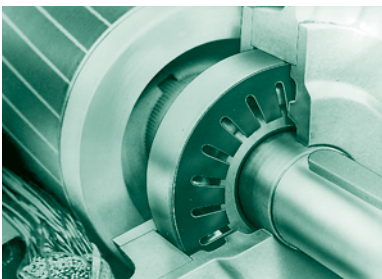
Installation site of a cb ball-bearing disc spring.
