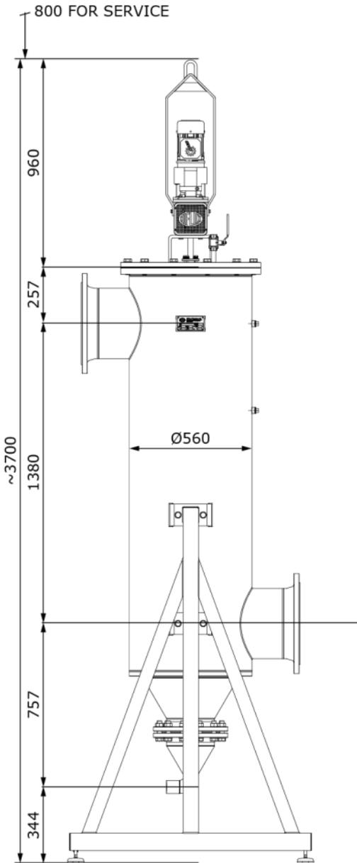
HiFlux Auto-line filters are manufactured from stainless acid-proof EN 1.4404 steel. The filter meets current standards and norms for pressure vessels, complies with the EMC directive and is CE labelled. The VLR-E filter is available ready for installation, complete with electronic controller and automatic drain-valve.
