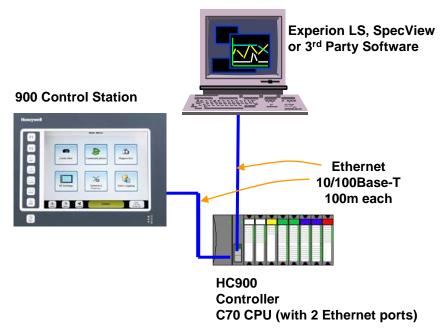
Use shielded CAT5 cable with RJ45 connectors. Connect to HC 900 to E2 of the C70 CPU and connect the host PC to E1.
