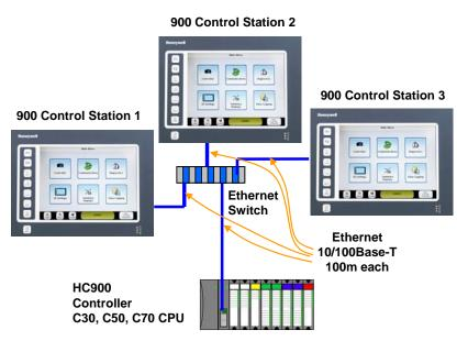
Up to 3 Control Stations may be connected to a HC900 controller using Ethernet. Multiple stations via RS 485 are not supported.
