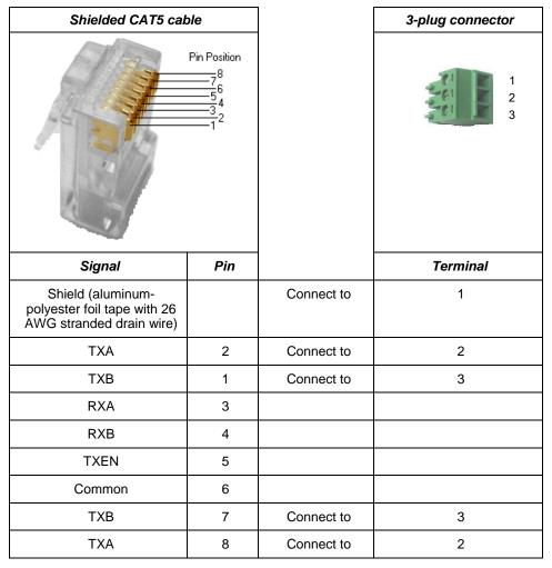
3. Cut off any unused wires in the cable and insulate with heat shrink tubing or other appropriate insulating material.
