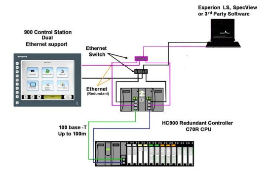
Connect to C70R using dual Ethernet cables.
