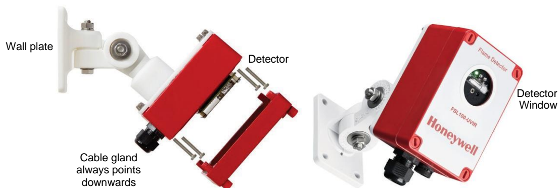
Figure 16. Swivel Mounting Fitment (Optional)
