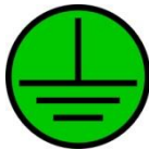
Figure 3. Protective Earth (Ground) Point
