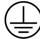
Figure 4. Equipment Earth (Ground) Point
