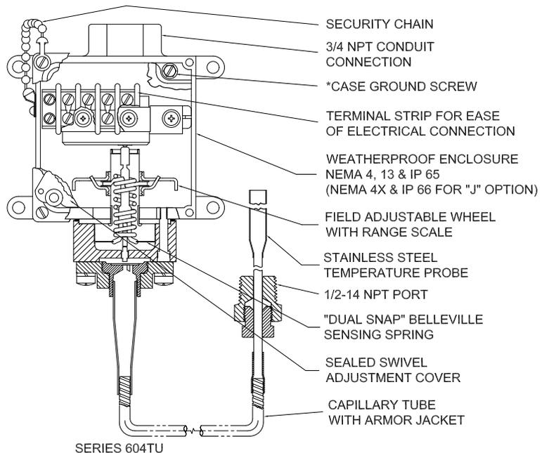
**FIELD SETTING:** Remove access cover. Adjust wheel as illustrated. Clockwise to increase settings. Counterclockwise to decrease settings.
