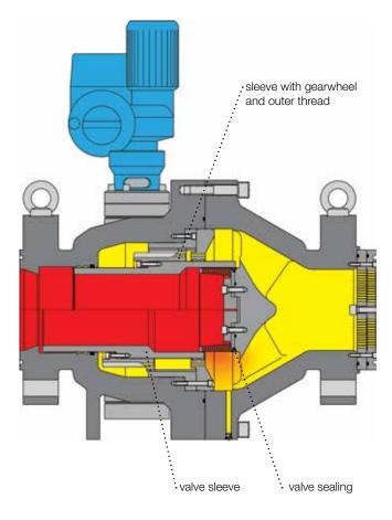
The flow control valves starting from inlet pipe dia. DN 200 and upward are designed for axial flow, and therefore a safety shut-off valve cannot be included. The proven valve sleeve system is used, thus enabling complete inlet and outlet pressure compensation. The valve sealing situated in the valve cone guarantees bubble-tight shut-off of the device.
