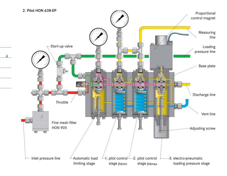
The pneumatic pilot control stages pdmin and pdmax automatically monitor the configured limit values. As soon as the equipment gets close to these limit values during operation, the pilot control stages are activated and keep the outlet pressure constant. Transition between the electro-pneumatic loading pressure stage controlled by the electronic controller and pressure limiting by the pilot control stages is effected independently and without jolts in both directions.
