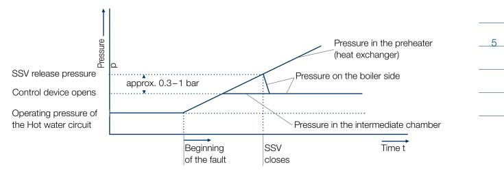
The safety shut-off device (SSV) then opens again if the pressure in the heat exchanger (above the valve plate) is brought to a value below the release pressure of the control device (SSV release pressure minus 0.3 to 1 bar). The remote indication is available in two different versions depending on the temperature in the hot water circuit; it cannot be retrofitted up to DN 200.
