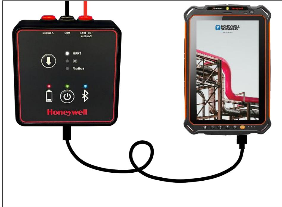
Figure 2-3: USB communication to the tablet
