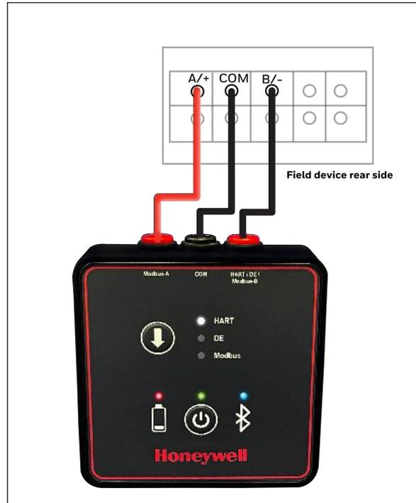
Figure 3-2: Connect to the Modbus field devices
