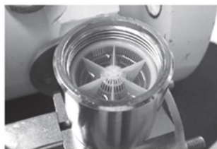
Fig. 6 | Oil supply tank
