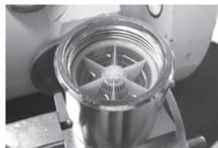
Fig. 5 | Oil supply tank
